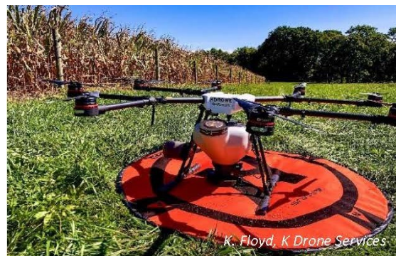
DJI drone equipped with hopper and spin spreader.
